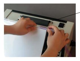
Manually turn your coil into the book. This is a very easy process. (Tip: It will be much easier to twist the front end of coils)
